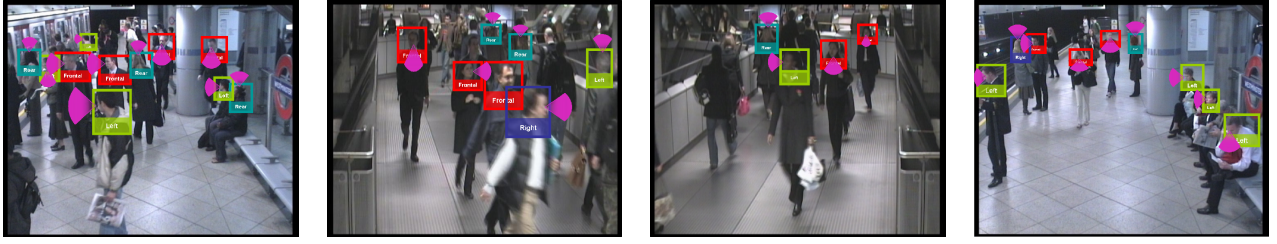
Figure 6: Examples of upper-body detection and pose estimation for body and head when the precision and recall rates are 0.802 and 0.383 respectively. Bounding box colour and text indicate body pose and magenta dials indicate head pose.
