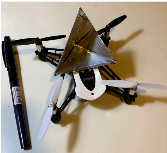
Fig. 6. Parrot Mambo Minidrone, with a trihedral retro-reflector for the RCS, for increased RF detectability.
