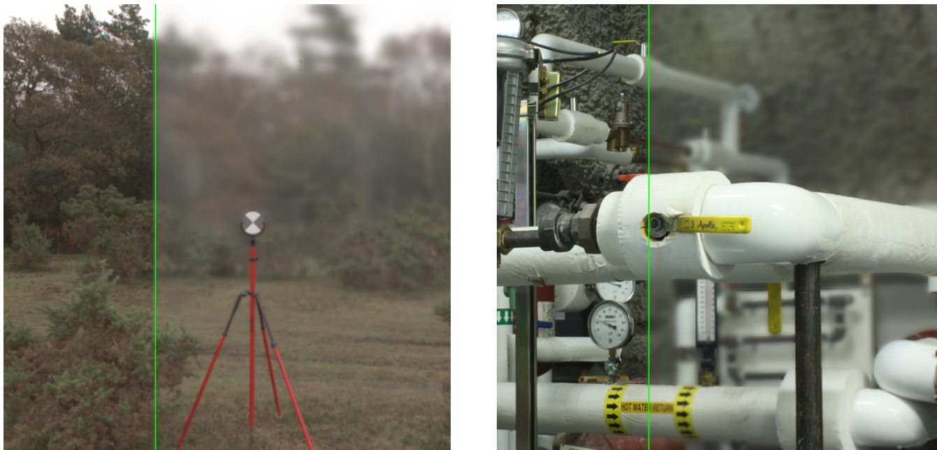
Figure 1: Synthetic haze effects have been automatically added to the right two-thirds of each image, based on the associated depth maps. There is a realistic loss of contrast and sharpness, in the distant parts of each scene, owing to synthetic absorption and scattering effects. Note that the closest objects remain clearly visible. These effects can be computed in real time, by 2D inhomogeneous diffusion, in a GPU shader.
