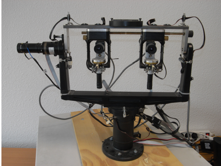
Figure 1: The POPEYE active binocular robotic head (designed and built in the Institute for Systems & Robotics, University of Coimbra, Portugal). The binocular vergence is controlled by a pair of motors, one below each camera. The pan and tilt angles of the head are controlled by another pair of motors.
