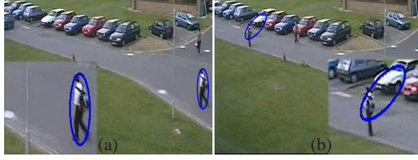
Figure 2: Example of wrong track using colour histograms.
